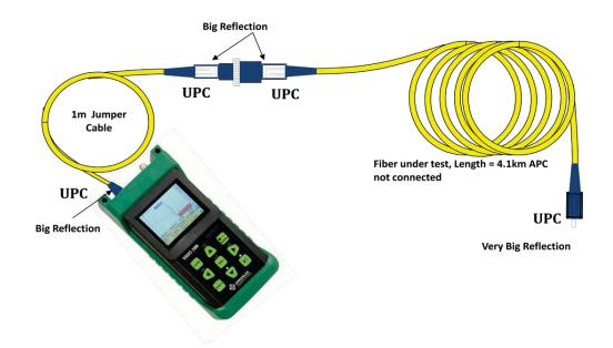
Mated UPC connections have high reflectivity (~45dB) An open (not connected) UPC will have a very high reflectivity (~14dB)
