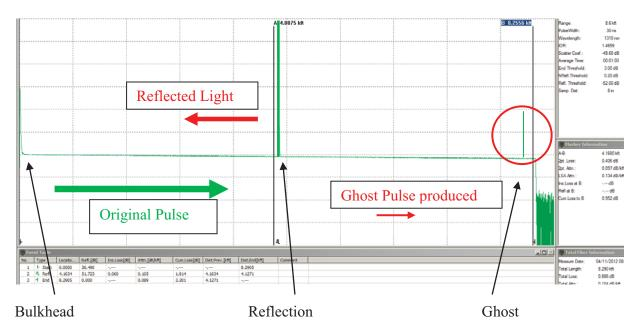
If there was a high reflection at the bulkhead there would be an immediate ghost produced. The effect of ghosting can be reduced if the reflection from the bulkhead is minimized.
